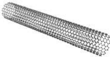
Figure 3.1a Schematic of a single-walled carbon nanotube (SWNT)
